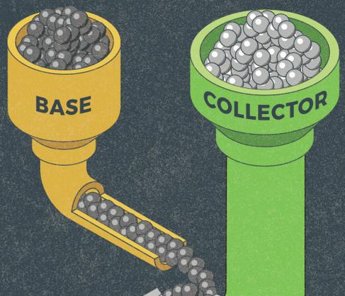
Sufficient pressure (current) flowing from the **BASE** allows electrons to flow from the **COLLECTOR** to the **EMITTER**, and to ground.
