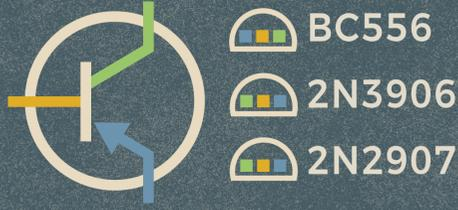
With a PNP transistor, voltage from the **EMITTER** will naturally flow to the collector unless there is sufficient current flowing from the **BASE**.
